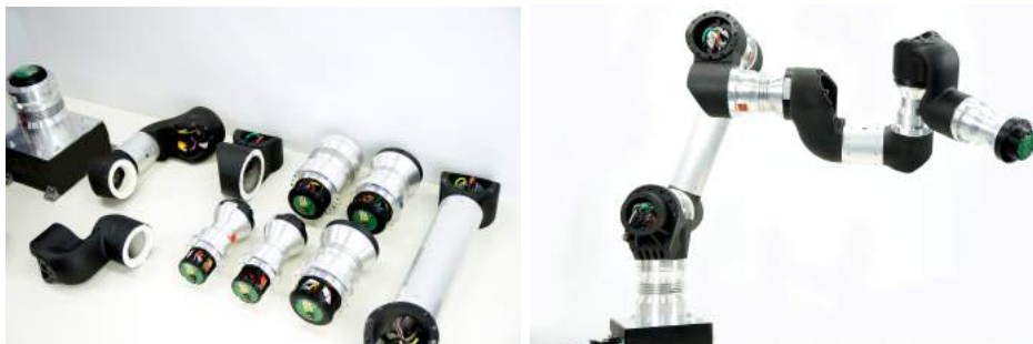
Figure 1: left: one pool of robot modules, which can be assembled to various robot compositions; right: one possible robot composition out of the set on the left.
