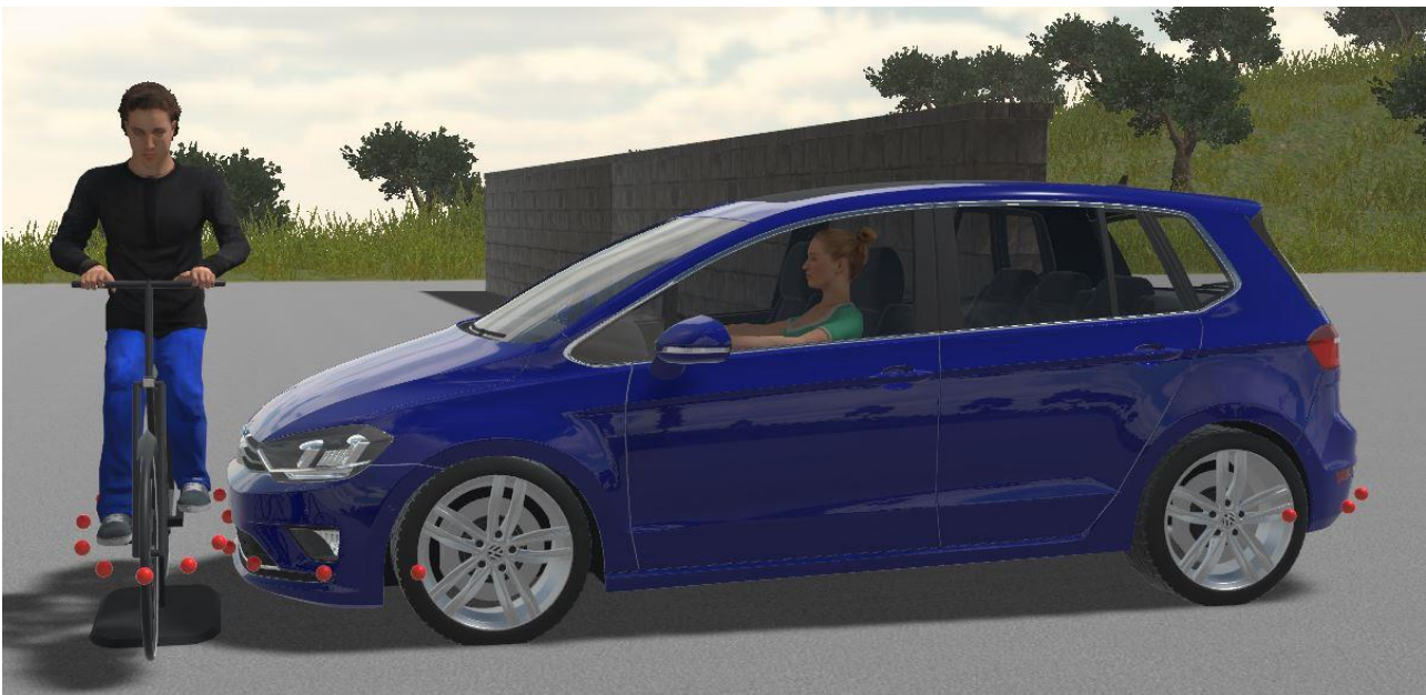
Simulation of an NCAP maneuver to test Automatic Emergency Braking (AEB) algorithms in DYNA4
